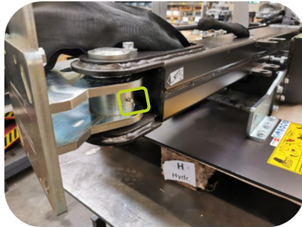
Grease-nipple on the swingarm, at the bracket for the attachment tool.
