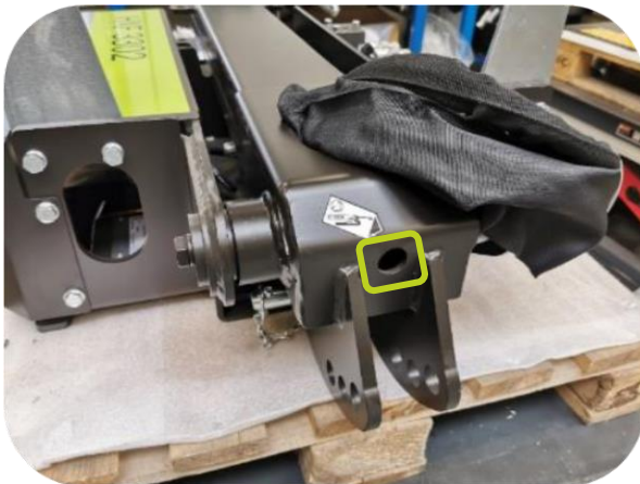
Grease-nipple on the inside of the swingarm: HXF multi carrier
