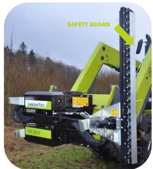
HXF multi carrier mounted with HL cutterbar in transport position. the attachment tool is facing inwards towards the vehicle, with safety guards on the blades for maximum traffic safety.
